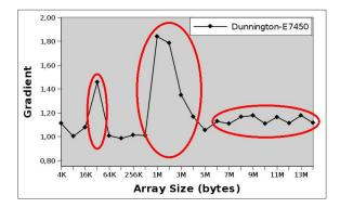
$L1 = 32KB\checkmark$  $L2 = 3MB\checkmark$  $L3 = 12MB\checkmark$
